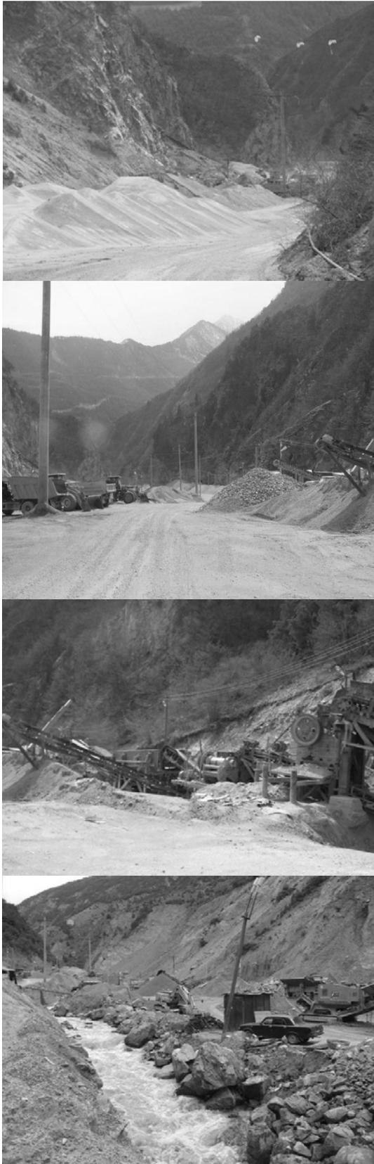
Photo 4. Stone-crushing plant on the river Sadon - the left tributary river Ardon (dumps along the river; the turbidity of river discharge waste technical water)
